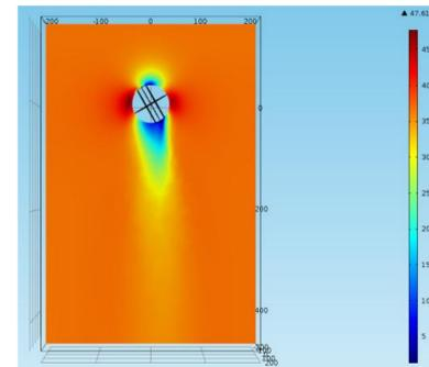
Figure 7. Velocity magnitude plot for a still ball at a seam angle of 20°
