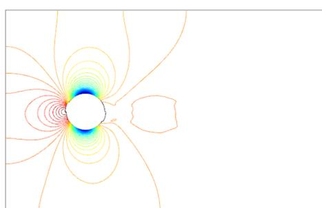
Figure 5. Pressure contour plot for 2D model
