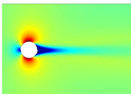
Figure 4. Velocity magnitude plot for 2D model
