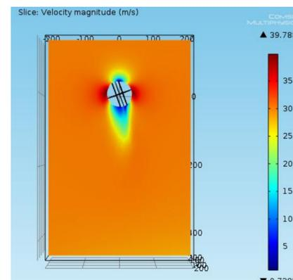
Figure 9. Velocity magnitude plot showing the flow profile for a ball velocity of 67mph, seam angle of 20° and backspin rate of 11.4 rev/s
