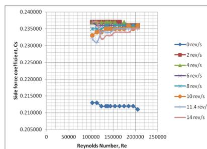
Figure 10. Graph showing the variation of the side force coefficient for varying backspin rates for a seam angle of 20°
