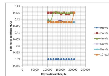
Figure 11. Graph showing the variation of the side force coefficient for varying backspin rates for a seam angle of 20°
