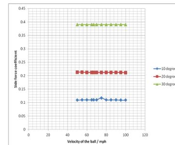
Figure 8. Graph showing the variation of the side force coefficient for differing velocities and seam angles
