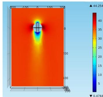
Figure 6. Velocity magnitude plot for a still ball at a seam angle of 0°
