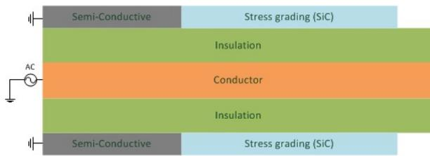
**Figure 1:** Insulation Arrangement of Endturn in stator winding.
