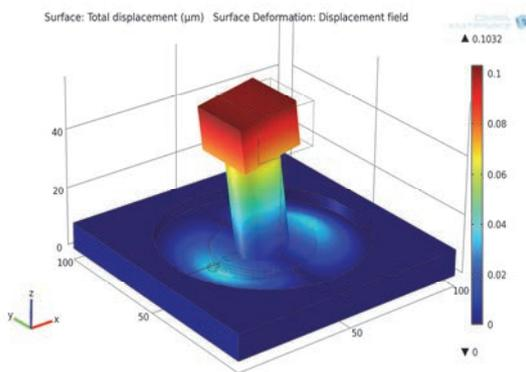
**Figure 6:** Displacement due to Electrostatic Force in 3D model
