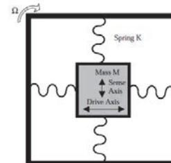
**Figure 1:** Basic Vibrational Gyroscope
